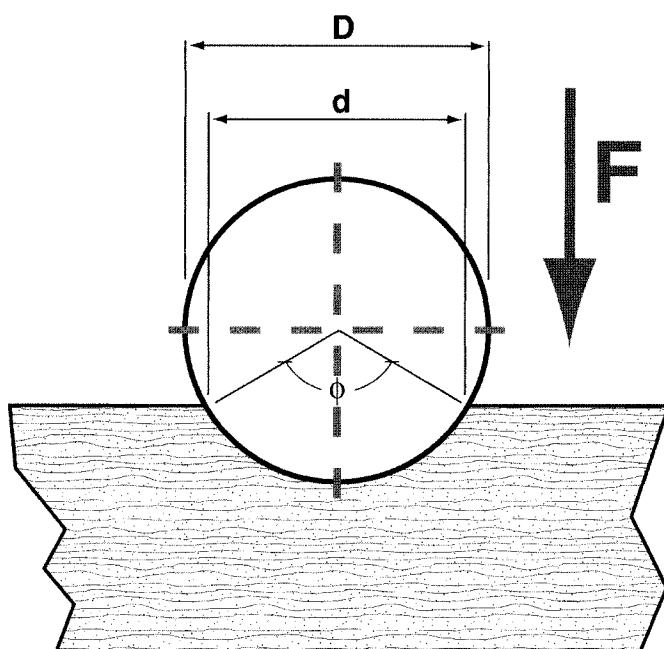
FIG. 1.—Test configuration of the modified Brinell firmness test. The parameters used to calculate the force exerted by the substrate are the diameter of the indentor (D), and the diameter of the impression (d).
