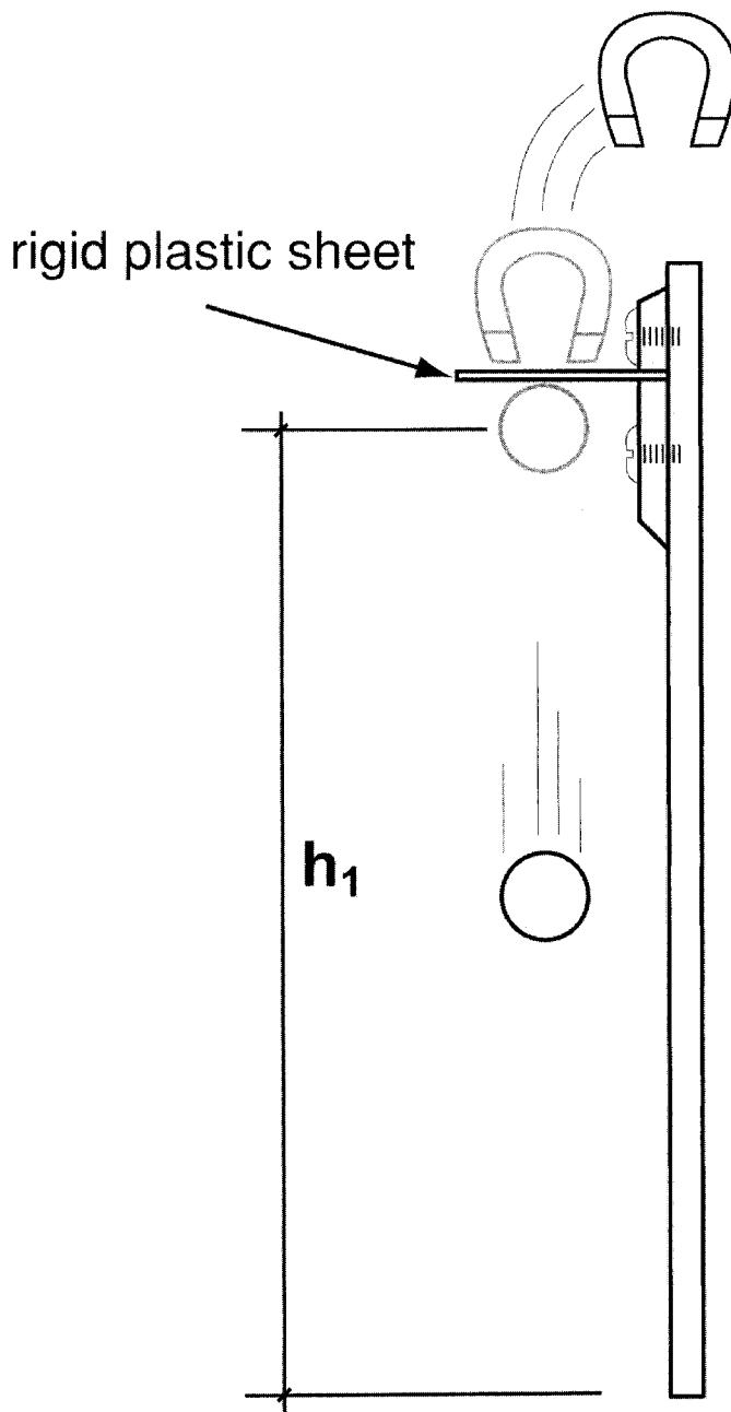
FIG. 3.—Modified Brinell test with magnetic release apparatus.
