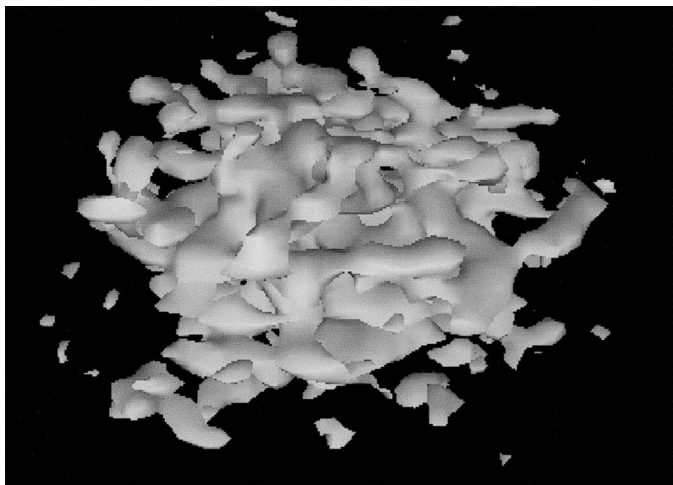
FIG. 5.—Three-dimensional surface rendering of the higher MRI signal. The signal roughly correlates to porosity zones of 12% and higher. Note the complexity and interwoven nature shown by the burrow interrelationships. The burrows appear to occupy much of the volumetric space available in the sediment block.
